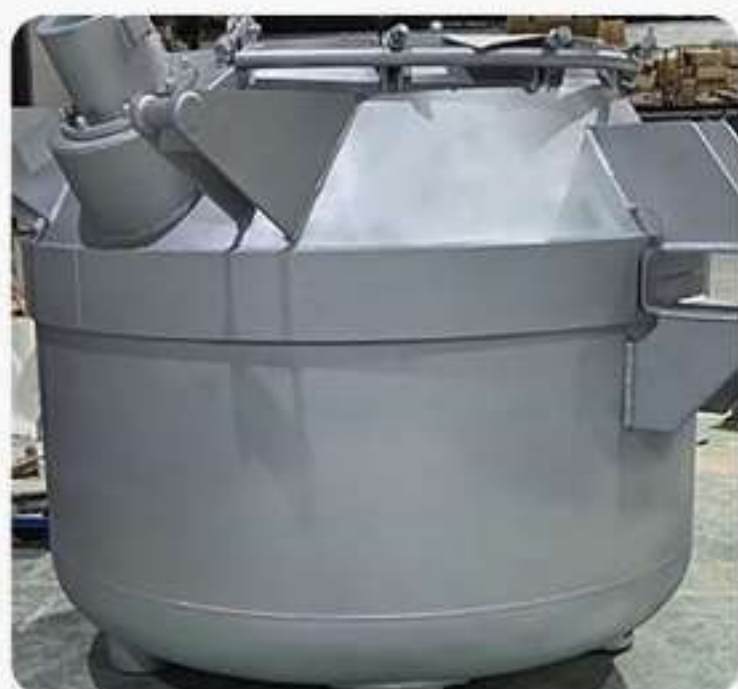
Holding Furnace & Transfer System
